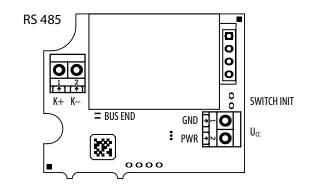
GND, PWR – Uccsupply voltage K+/K– – communication line BUS END – RS 485 termination
