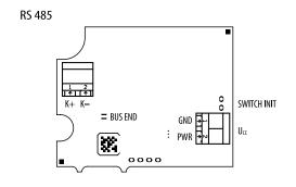
GND, PWR –  $U_{cc}$  supply voltage K+/K- – communication line BUS END – RS 485 termination
